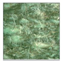
**Fig. 10:** Mould on test specimen 122 (H41), 40-fold enlargement.
