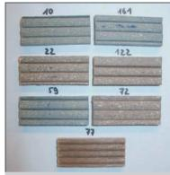
Fig. 3: Selected test specimens after the mould test: no vegetation macroscopically detectable.
