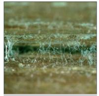
Fig. 9: Mould on test specimen 77 (Bangkirai), 50-fold enlargement.
