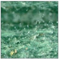
**Fig. 5:** Mould on test specimen 10 (H40), 40-fold enlargement.
