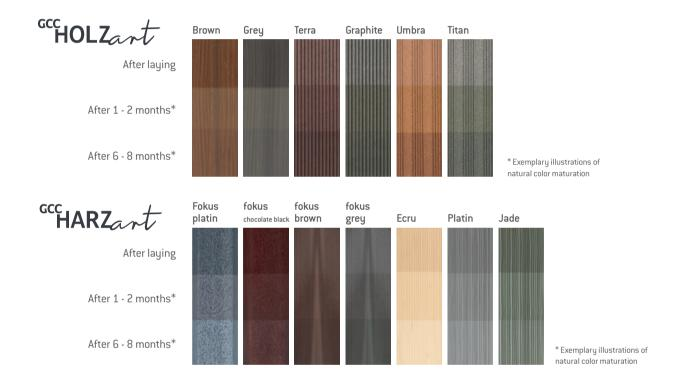
The natural colour maturation is tested in the accelerated weathering tester. Hereby, the solar radiation and humidity are simulated in periodic changes, 1000 hours of weathering correspond to around one year of outdoor weathering.
